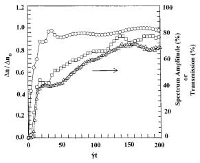
**Figure 5.** Variations of  $\Delta n^+(t,\dot{\gamma})$  (O),  $A_{\rm s}^+(t,\dot{\gamma})$  (D), and transmission ( $\triangle$ ), with  $\dot{\gamma}t$  for PSHQ10 at  $\dot{\gamma}=0.3~{\rm s}^{-1}$  and  $T_{\rm NI}-30~{\rm ^{\circ}C}$ .
