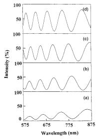
**Figure 2.** Transmission spectra for PSHQ10 during shear start-up with measurements taken at (a) 9, (b) 18, (c) 72, and (d) 216 strain units, with  $\dot{\gamma}=0.3~{\rm s}^{-1}$  and at  $T_{\rm NI}=30~{\rm c}$ C. For each trace, the intensity data are expressed as a percentage of the light transmitted by the polymer in the isotropic phase. Incident light is polarized at an angle 45° to the flow axis and the analyzer is parallel to the polarizer.
