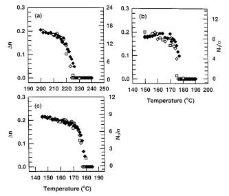
**Figure 9.** Temperature dependence of steady-state birefringence  $\Delta n$  at  $\dot{\gamma}=0.05~{\rm s}^{-1}$  in the heating ( $\blacklozenge$ ) and cooling processes ( $\diamondsuit$ ) and temperature dependence of steady-state stress ratio  $N_1/\sigma$  at  $\dot{\gamma}=0.05~{\rm s}^{-1}$  ( $\square$ ) for (a) PEHQ10, (b) PTHQ10, and (c) PSHQ10.
