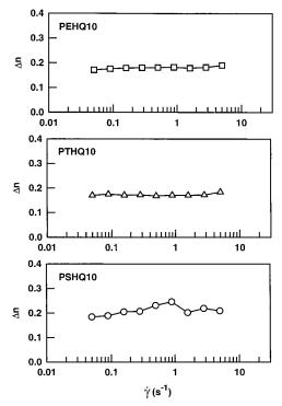
**Figure 6.** Plots of  $\Delta n$  versus  $\dot{\gamma}$  in steady-state shear flow for  $(\Box)$  PEHQ10,  $(\triangle)$  PTHQ10, and  $(\bigcirc)$  PSHQ10 at  $T_{\rm NI}-30$  °C.
