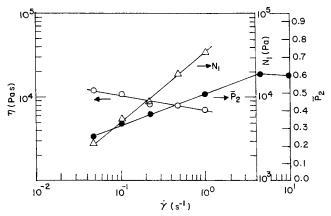
**Figure 11.** Shear rate dependence of viscosity  $\eta$  ( $\bigcirc$ ), first normal stress difference  $N_1$  ( $\triangle$ ), and bulk orientation order parameter  $P_2$  ( $\bullet$ ) in steady-state shear flow of PSHQ10 at 160  $^{\circ}$ C.  $P_2$  was determined from X-ray scattering, which corresponds to the bulk orientation order parameter S defined by eq 5.
