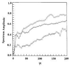
**Figure 4.** Variations of normalized spectrum amplitude  $A_s^+$ - $(t,\dot{\gamma})$ , computed from the amplitude of the FFT power spectrum of the transmitted intensity, with  $\dot{\gamma}t$  upon startup of shear flow for ( $\Box$ ) PEHQ10, ( $\triangle$ ) PTHQ10, and ( $\bigcirc$ ) PSHQ10 at  $\dot{\gamma}=0.3~{\rm s}^{-1}$  and  $T_{\rm NI}-30~{\rm °C}$ .
