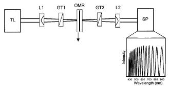
**Figure 1.** Schematic of the optical train used to measure flow-induced birefringence of thin, heated polymer films. White Light (TL) is focused on the sample shearing plane (OMR), using a lens (L1), and polarized (GT1) at an angle 45° from the flow axis. Light then passes through an analyzer (GT2) parallel with the polarizer and collected with a lens (L2) to a spectrometer (SP).
