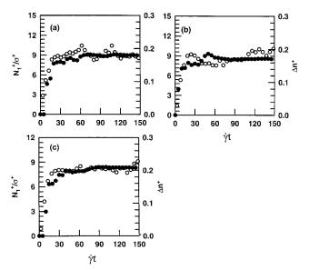
**Figure 8.** Plots of  $N_1^+(t,\dot{\gamma})/\sigma^+(t,\dot{\gamma})$  versus  $\dot{\gamma}t$  ( $\bigcirc$ ) and  $\Delta n^+(t,\dot{\gamma})$  versus  $\dot{\gamma}t$  ( $\bigcirc$ ) upon startup of shear flow at  $\dot{\gamma}=0.3$  s<sup>-1</sup> and  $T_{\rm NI}-30$  °C for (a) PEHQ10, (b) PTHQ10, and (c) PSHQ10.
