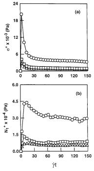
**Figure 7.** (a) Variations of  $\sigma^+(t,\dot{\gamma})$  with  $\dot{\gamma}t$  and (b) variations of  $N_1^+(t,\dot{\gamma})$  with  $\dot{\gamma}t$  upon startup of shear flow at  $\dot{\gamma}=0.3~\text{s}^{-1}$  and  $T_{\text{NI}}-30~\text{°C}$  for ( $\square$ ) PEHQ10, ( $\triangle$ ) PTHQ10, and ( $\bigcirc$ ) PSHQ10.
